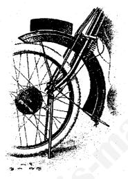
Removing Front Wheel— Disconnect cable yoke and from brake operating lever, remove anchor plate bolt from fork end, and after slackening off spindle muts the wheel will then fall out of slots in fork ends.
