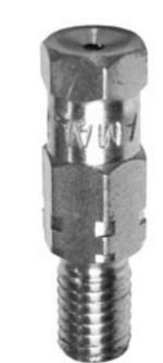
THROTTLE ADJUSTING SCREW (26). Set this screw to hold the throttle open sufficiently to keep the engine running when the twist grip is off. An "O" ring is fitted to the screw to hold this adjustment by friction.
